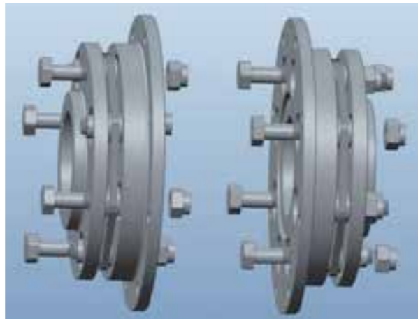
Diagram for couplings series HNS-RH
