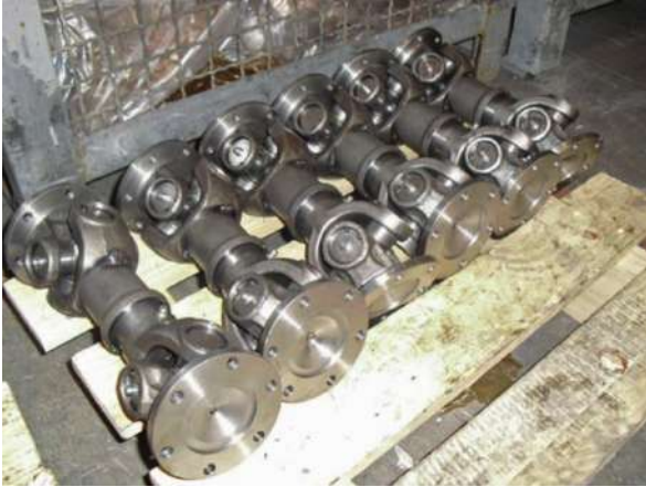
Cardani DNFx 100 C extracorti Universal shafts DNFx 100 short design
